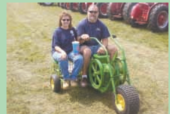
Two-seater Deere mini bike (above and below) combines a Heald mini bike frame with a "hit and miss" Deere engine.
