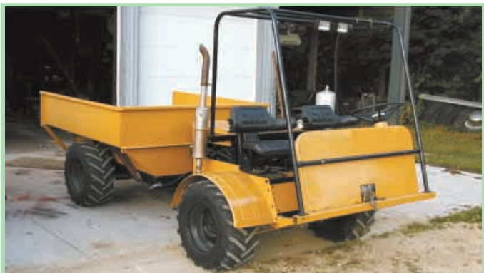
Kerry Tamke calls this home-built, articulated, 4-WD utility vehicle the "Pugster".
