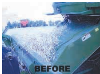
Canvas covers top of feederhouse at a steep enough slant so debris slides back into header.
