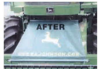
Canvas covers top of feederhouse at a steep enough slant so debris slides back into header.
