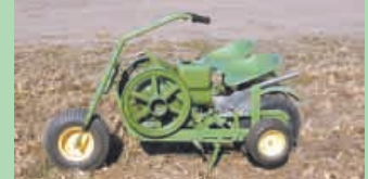
Two-seater Deere mini bike (above and below) combines a Heald mini bike frame with a "hit and miss" Deere engine.
