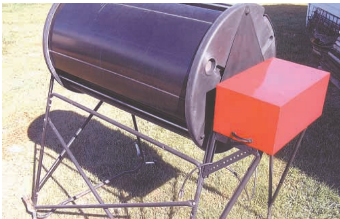
Using an electric motor controlled by a timer, James Novacek rotates the drum automatically on his Garden Ways E-Z spin composter.
