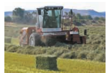
Freeman Baler is powered by a fuel-efficient 115 hp Deere engine and has a new spacious cab.
