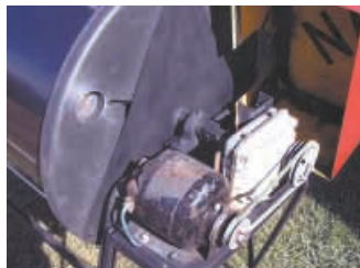
Motor and gear reduction box mount on a metal frame attached to composter stand.
