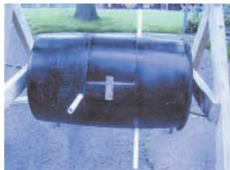
Two pieces of pvc pipe serve as handles to make it easy to rotate the barrel.
