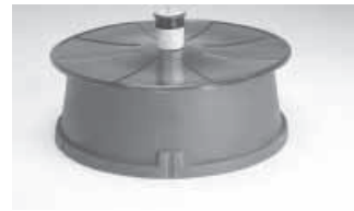
Metal reservoir mounts on feeder's cover and holds liquid insecticide, which wicks down to saturate a layer of felt on cover's bottom side. As animal sticks its nose under cover to get at mineral, its head brushes against felt and gets covered with insecticide.
