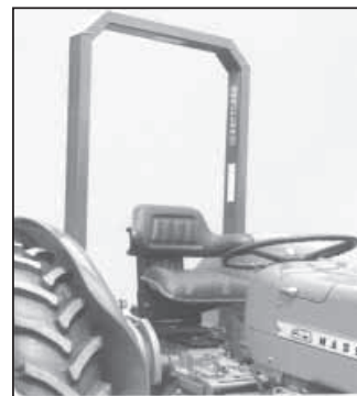
Hercules E-Z Fit ROPS are designed for tractors made from 1939 to 1985 that weigh 7,000 lbs. or less.
