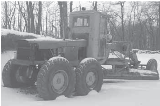
Rodney Baker repowered this old road grader with a 6.2-liter diesel engine and a 3-speed automatic transmission out of a 1984 Chevrolet 3/4-ton pickup.
