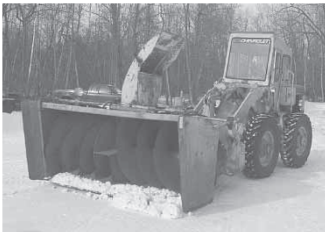
He also repowered an old Hough end loader. A snowblower powered by a Chevrolet 350 cc engine and 4-speed transmission can be quick-tached to the bucket.
