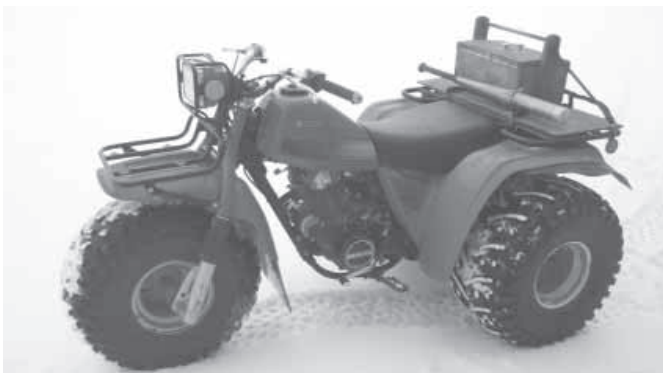
"It has a much shorter turning radius than a quad, and also costs less," says Keith Schole about his 1982 Honda 3-wheeler. He uses it during calving time.
