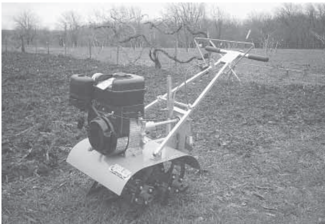
"It's so well balanced that a 12-year-old can operate it," says Roy Huber about his rototiller. The front tines rotate forward and the rear tines rotate backward.
