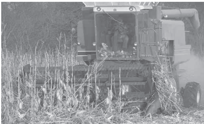
LeRoy Lyne took the reel off a 15-ft. flexhead and mounted it on his 6-row, 30-in. Deere corn header. "The reel works like a brush. It pulls corn stalks off the snouts and feeds them into the combine," he says.
