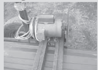
Saw is powered by an electric motor that has a 16-in. blade bolted to it. Motor is bolted to a metal carriage that rides between a pair of channel iron guides.
