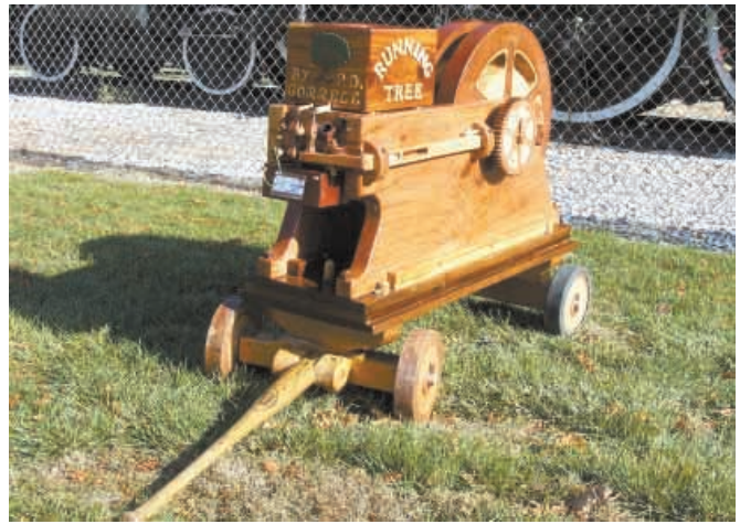
There are no metal parts in Gorrell's engine, which was made from 8 kinds of wood.
