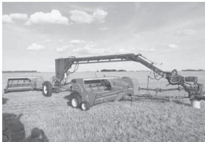
Dwayne Archer designed a hitch that lets him pull two balers at a time (above). Oil from a pto-driven hydraulic pump powers 55 hp hydraulic motors at each baler hookup point.
