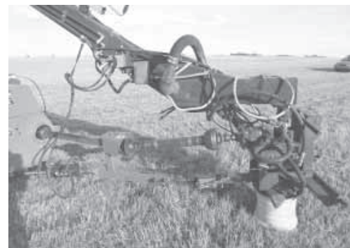
Dwayne Archer designed a hitch that lets him pull two balers at a time (above). Oil from a pto-driven hydraulic pump powers 55 hp hydraulic motors at each baler hookup point.
