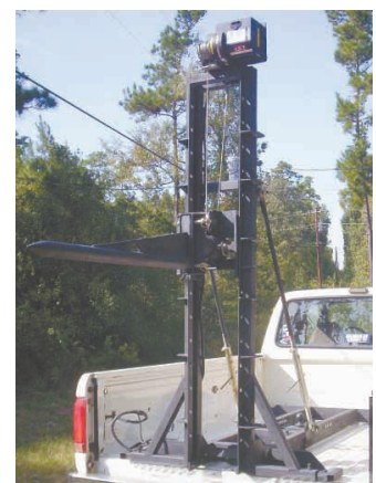
Lift mechanism has an electric winch operated by a toggle switch in cab.
