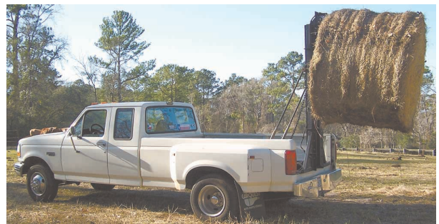
"As far as I know it's the only pickup bale mover designed to raise and lower the bale straight up," says Brady Brooks about his new single-bale mover.
