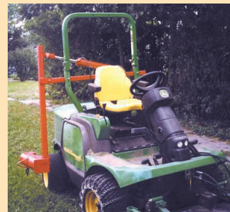
Pushing on the lever extends the cylinder to drop the counterweight straight down alongside the mower.
