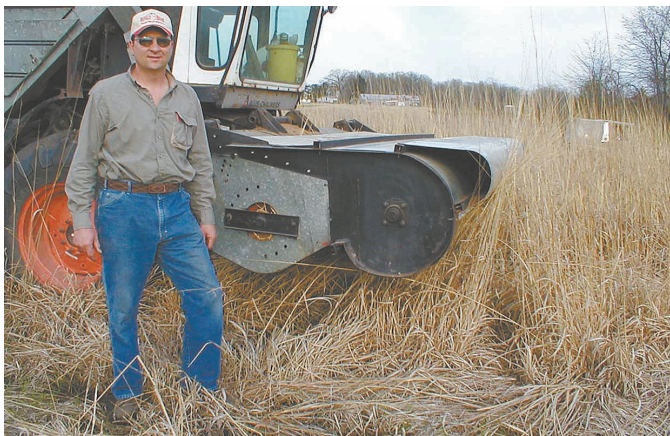
Faced with a heavy crop of native grass seed, Wallace White built this custom stripper header for his older, small combine. It strips seed off the stems to reduce plant debris.
