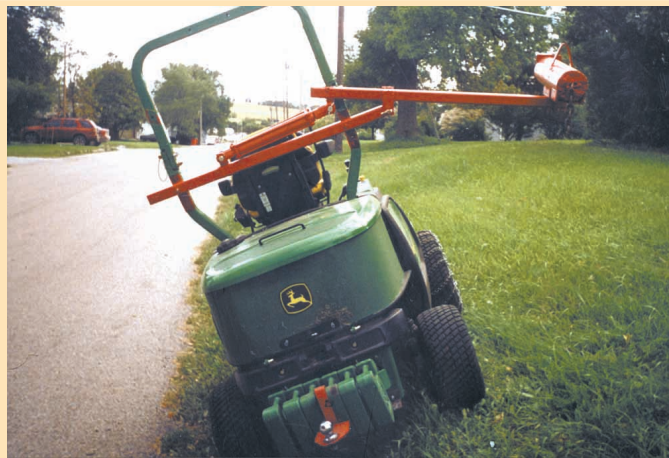
Elmer Pinkerton built this 150-lb. counterweight to hold his Deere mower stable on slopes. Pulling on a lever retracts a hydraulic cylinder to bring counterweight to a nearly horizontal position, keeping mower from tipping over on hillsides.
