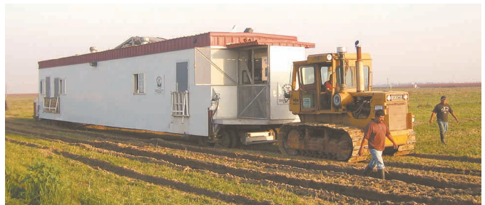
Once a week, Mark McAfee rotates his milking parlor as he rotates his cows through a series of paddocks. It looks like a 65-ft. mobile home, but it weighs 55,000 lbs.
