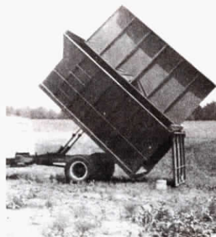
Edwin Scott's truck lid consists of a welded tube frame coated with neoprene-coated nylon.
