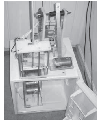
The remote control activates a small elevator that lifts one can at a time through a hole in the top of the fridge and loads it into a catapult arm. A second click fires the can through the air.
