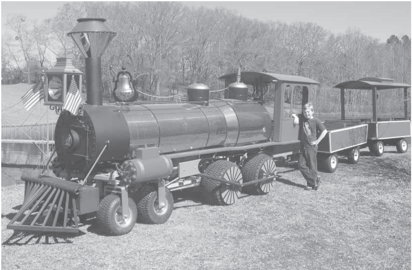
Rubber-tired locomotive was built from components off a pair of junked pecan sweepers. It pulls a 4-wheeled car and caboose that can hold up to 12 kids at a time.
