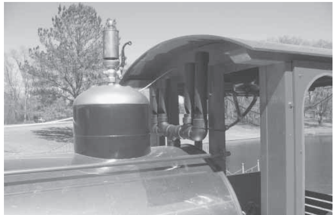
An air compressor that's belt-driven off the engine supplies air for the locomotive's whistle. It's made out of four 1 1/2-in. dia. pvc pipes of different lengths to provide the right sound.
