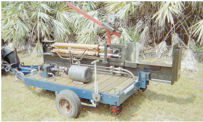
Log splitter is powered by a 5 hp, 3-phase electric motor so it's quiet and produces no exhaust fumes.
