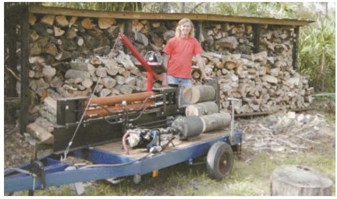
A boom fitted with an electric winch swings log onto splitter from any direction.
