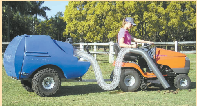
Paddock Vac vacuum works on dry or wet manure and doesn't pick up small surface items such as rocks.
