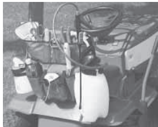
"Tractor Pac" tool holder hangs on back of tractor seat to hold a variety of tools.
