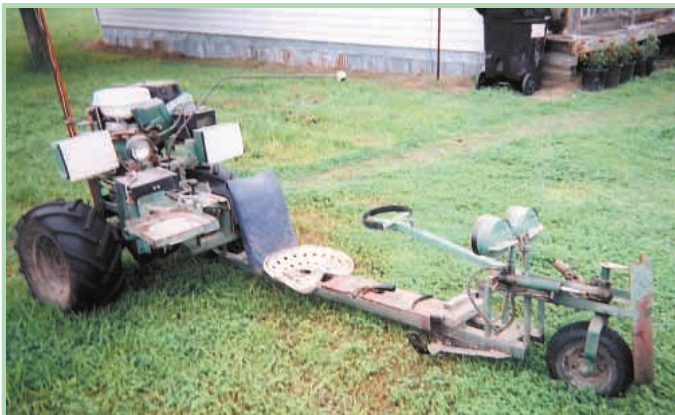
Marvin Niekamp cut apart a 16 hp Gilson lawn tractor to make this picking rig.
