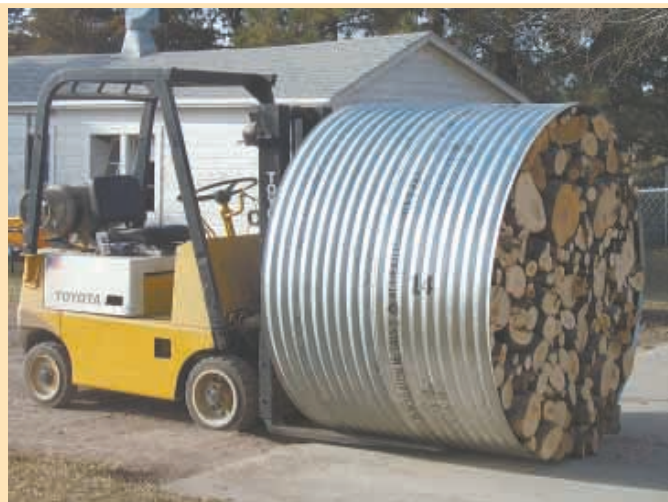
Tim Kelliher stores firewood inside 4-ft. long rings of 6-ft. dia. metal culvert. He uses his 3-pt. bale carrier or pallet forks to move the rings around.
