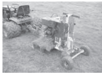
When folded up, mower is only 35 in. wide.
