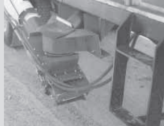
Inside the truck, a small hopper for bagged seed corn is located directly above auger (left). Photo at right shows how auger pivots back and forth.
