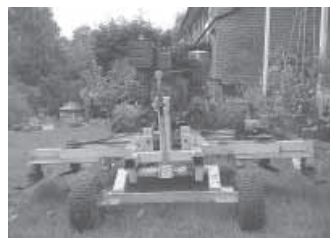
Mower is powered by a Briggs & Stratton 10 hp, single cylinder engine.
