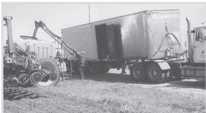
By equipping an enclosed semi trailer with a hydraulic auger, T.J. and Teddy Shambaugh can quickly fill large planter hoppers.
