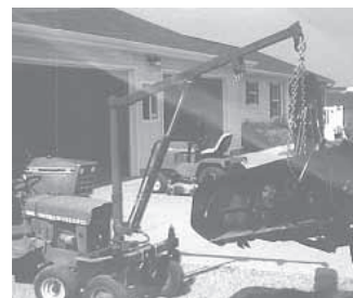
Two-wheeled, telescoping boom mounts on frame that's completely independent of tractor. It supports the boom and also balances the load.
