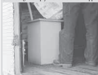
Inside the truck, a small hopper for bagged seed corn is located directly above auger (left). Photo at right shows how auger pivots back and forth.
