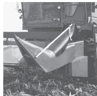
When opening a field, Rich Mahlow tilts the outside snout of his corn head upward so weeds and hidden objects along edge of field don't catch it and cause damage.
