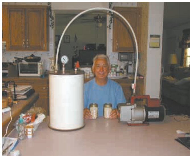
"My bulk food vacuum packing system gives me a seven-year-plus shelf life for dry goods," says inventor Danny Mizell.
