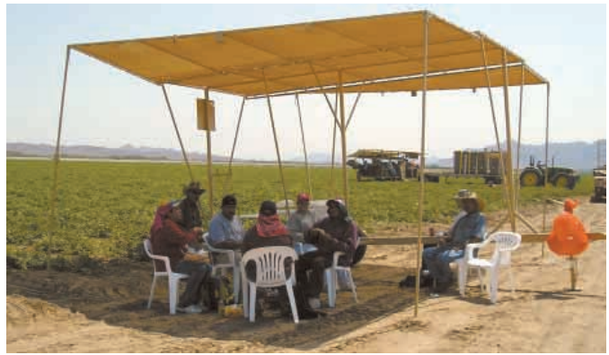
A California company builds these portable shade units to provide workers with a cooler, more comfortable place to take breaks. The two-wheeled, single axle trailer has three 8-ft. wide panels covered with "85 percent shade cloth".
