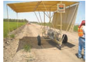
A California company builds these portable shade units to provide workers with a cooler, more comfortable place to take breaks. The two-wheeled, single axle trailer has three 8-ft. wide panels covered with "85 percent shade cloth".
