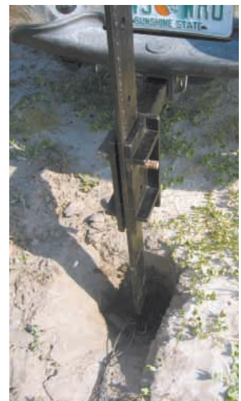
Pickup "plow" slides into receiver hitch, allowing you to bury lines fast and easy. It can dig down to 18 in. below grade.
