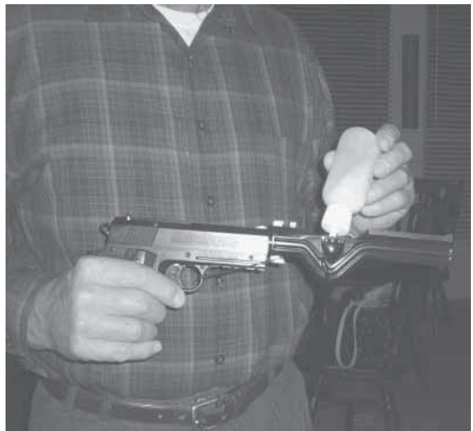
"If you can see 'em, you can shoot 'em," says Martin Jenson, inventor of the "Bugblaster" that turns an ordinary air gun into a mini "shotgun" that shoots table salt. Photo shows Bugblaster on a Crossman .357 CO2 air gun, which is made to look like a .357 Magnum.
