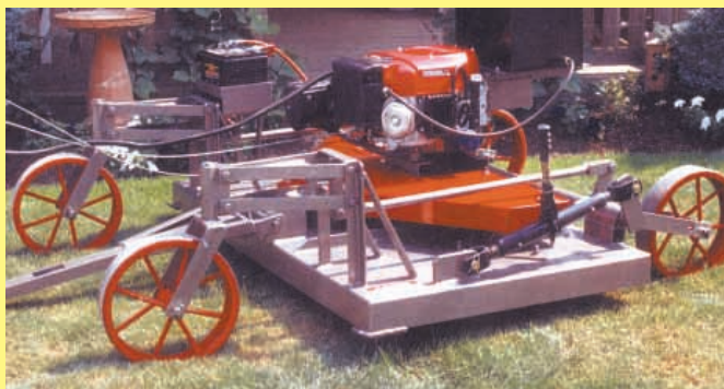
Trailing mower is designed for use with horses, ATV's, utility vehicles or non-pot equipped tractors. The heavy gauge deck mounts on steel wheels.
