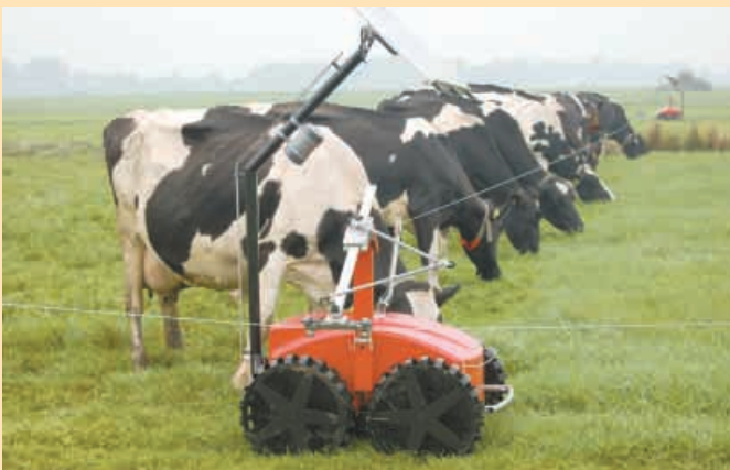
Automatic grazing system consists of two mobile robots powered by solar panels and connected to an electrified wire. Each day the operator can set how much pasture should be released, and the robots calculate when to move.
