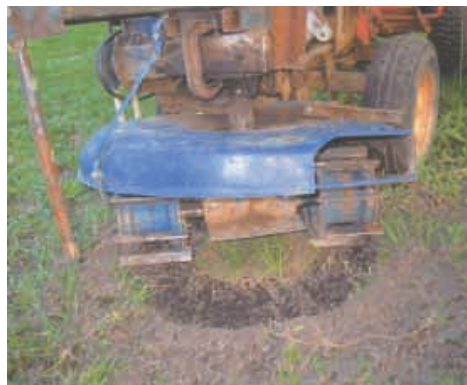
Reyenga earth grinder is designed to grind up weeds at ground level so weed seeds stay buried. It consists of two 12-in. dia. drums, with 1-in. high blades, mounted on a 22-in. shaft with a gearbox at the center.
