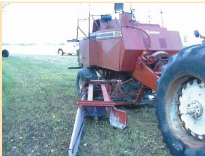
"Re-baler" is used after a field has been baled. It "packages" 12 small bales so they look and handle like one big bale.
