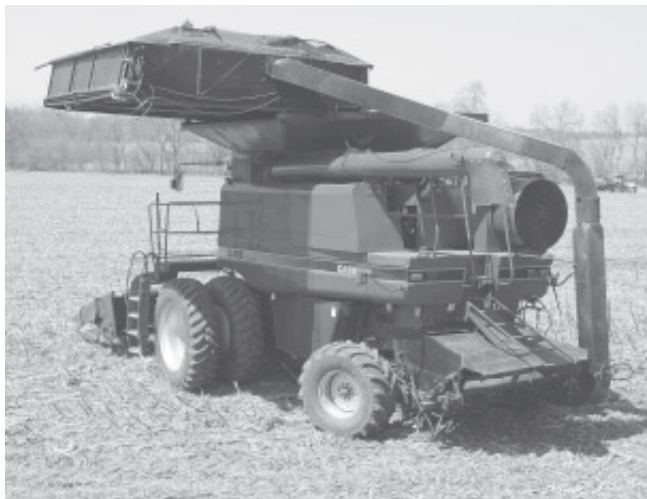
Material is blown up and over combine to a 320 cu. ft. storage basket that sits above combine's grain hopper.
