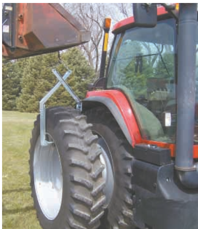
EZ Dual Changer is a scissors clamp that hangs from a chain hoist on front-end loader.
