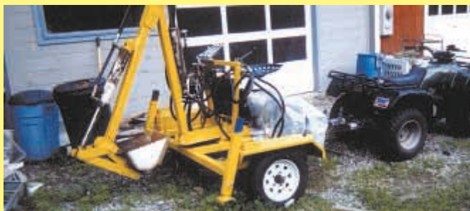
Gerrier's backhoe rides on a pair of 12-in. wheels and tows behind his ATV. Power is supplied by a 5 hp Honda gas engine with an 11 gpm pump.
