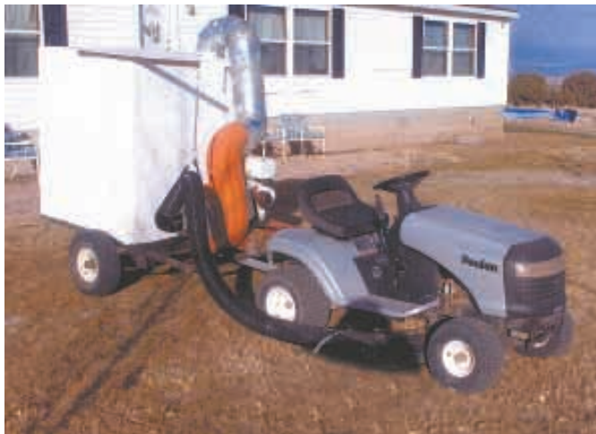
To build this leaf vacuum, Leonard Lilienthal dismantled a walk-behind vacuum and mounted its engine and blower assembly on a trailer, along with a plywood box.
