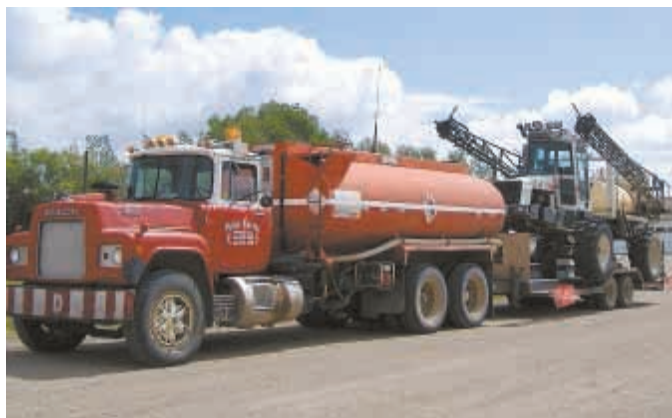
Muhr Farms assembled this water truck with used equipment including a 1981 Mack tandem, a 3,800-gal. water tank, and a truck wrecker pump.
