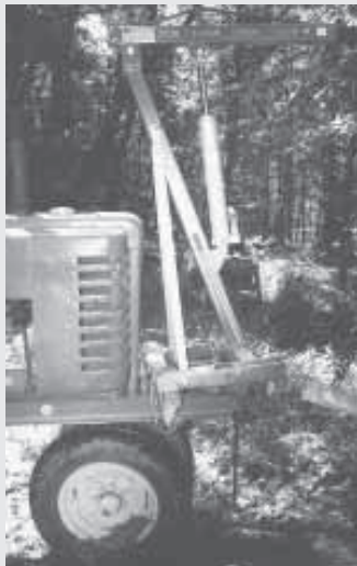
Woody Cone mounted this engine hoist on front of his older Deere tractor.
