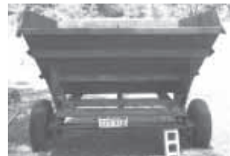
Wheeled dumpster mounts on an old house trailer axle with brakes and lights.
