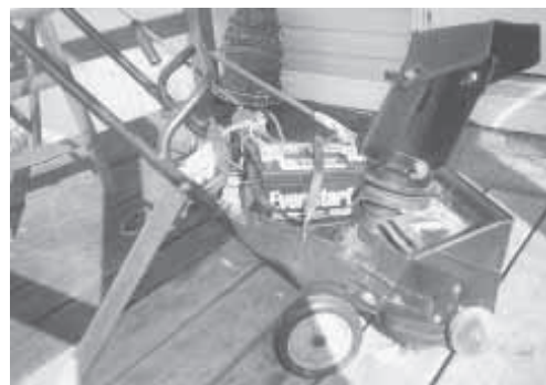
"I like it because there's no need to hassle with gas or electric cords," says John Gross, who converted his 2-cycle gas-powered snowblower to a cordless model.
