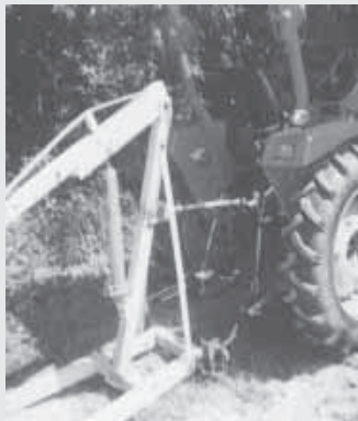
George Diggs removed the caster wheels from a shop hoist and mounted it on his tractor's 3-pt. hitch. "There seems to be no end to what I can use it for," he says.
