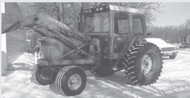
Wilbert Loewen modified a Massey 1135 cab and added it to his Deere 4020 tractor.
