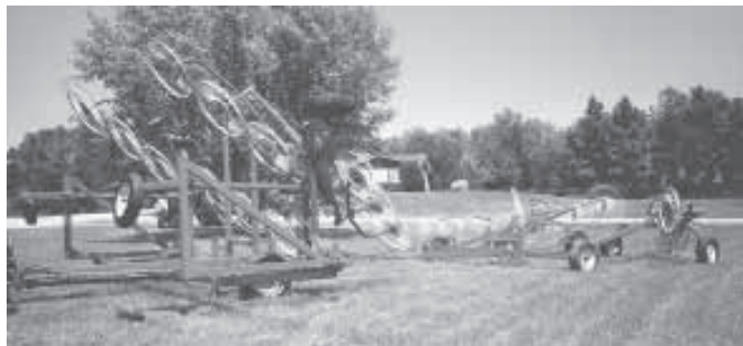
Raymond Janisch put four used Vicon rakes together to create this folding wheel rake.
