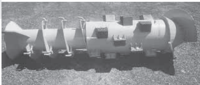
Fingers on the auger flighting are infinitely adjustable, making it easy to set the rotor for varying crop conditions.
