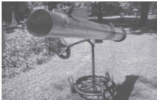
The main tube on Schraufnagel's telescope is made from a galvanized silo filler tube.
