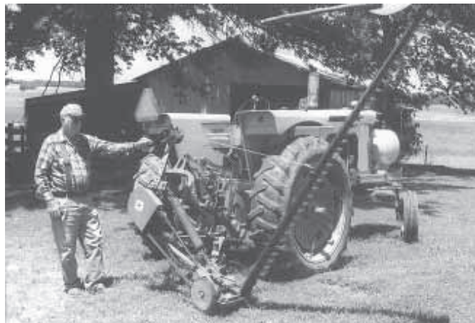
Boat winch mounts on mower frame. To raise sicklebar, Marley connects a cable to middle part of sicklebar and cranks the winch.
