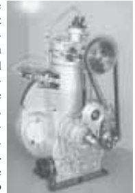
Heated air from the cylinder charges a combustion chamber as fuel is injected.
