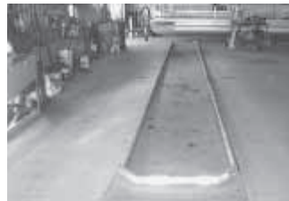
Auto pit cover can be opened or closed by simply pushing a button. Because the pit can be closed, dangerous fumes cannot settle into pit between uses.
