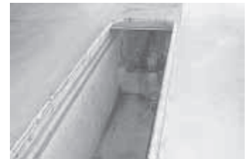
Auto pit cover can be opened or closed by simply pushing a button. Because the pit can be closed, dangerous fumes cannot settle into pit between uses.
