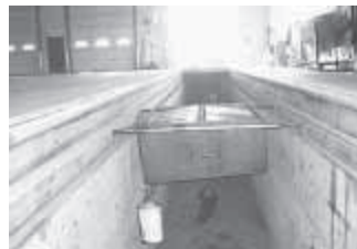
Door opener moves 10 4-ft. cover sections of 1/4-in. thick deck plate back and forth across top of pit. When rolling oil pan is full, Dorwin moves it to the end of the pit to dump.
