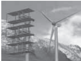
Instead of a spinning blade, the WindWing consists of horizontal blades that pivot up and down on levers that drive a generator.
