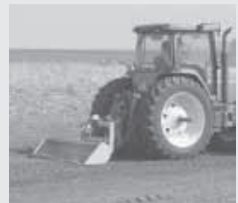
Rear-mounted bucket/blade has a deep mouth to catch and hold dirt as it's skimmed off.
