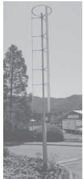
Windspire is a 30-ft. tall, 4-ft. dia. unit that spins in position. It comes with everything you need to plug it into the house or grid.
