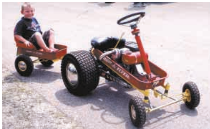
Matt and Ken Schindeldecker "self-propelled" a Radio Flyer toy wagon with a Honda 4 hp gas engine. Matt's 4-year-old son Brady rides in a smaller wagon.
