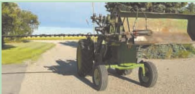
Hydraulic-powered, loader-mounted trimmer lets John Ivers shape up a hedge fast.
