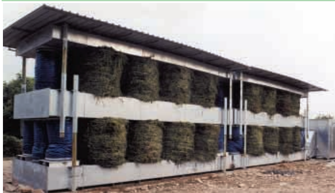
Bales are dried from the top and bottom at the same time.
