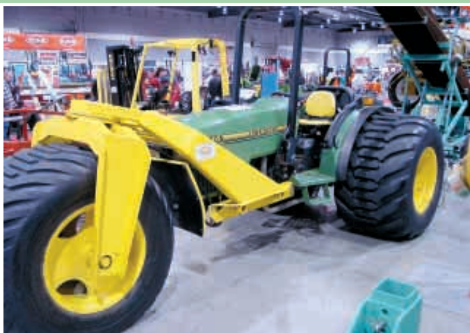
Large float wheels allow converted tractor to easily maneuver on soft ground.
