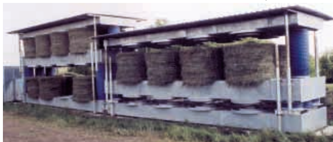
To load the bales, the top floor drops down to a height of 4 ft. for easy loading.
