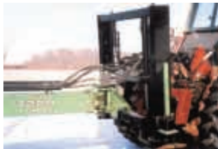
Planter hitches to moveable "drawbar" inside hitch frame.
