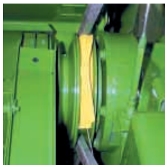
Drive belt tool simply derails belt to move it over the next pulley. It eliminates the need to loosen belt.
