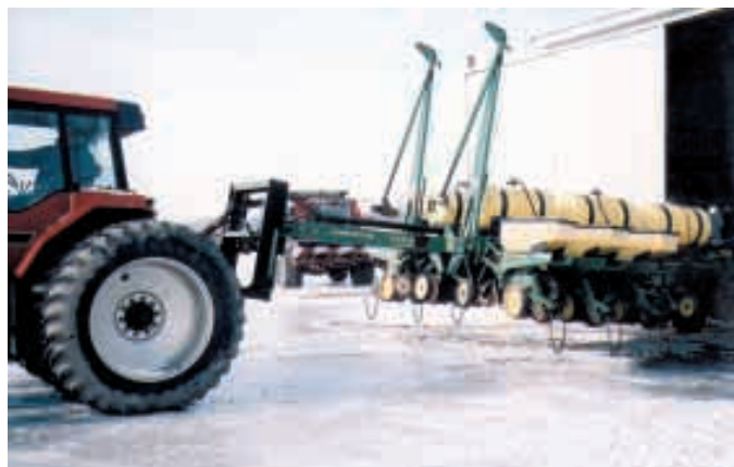
Extra 12 in. of height keeps planter from catching on ditches, railroad tracks, or other obstacles.
