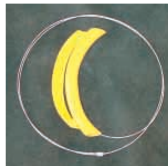
Drive belt tool simply derails belt to move it over the next pulley. It eliminates the need to loosen belt.
