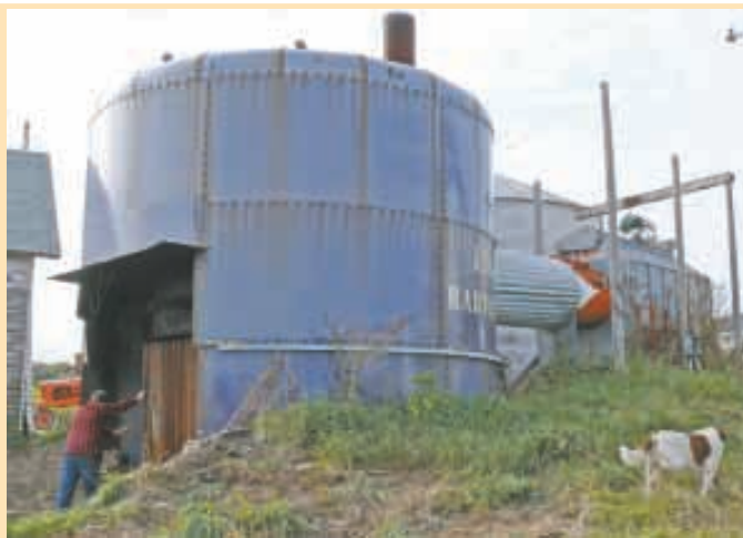
"It cut our fuel bill in half," says Craig Stortz, who built a bean stover-fired burner to dry corn.
