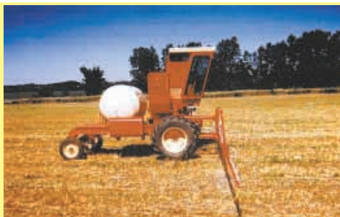
A 45-ft. long, 3-pt. mounted boom mounts in place of the header, while a 550-gal. tank mounts behind the cab.
