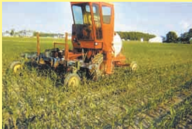
An anhydrous toolbar can be mounted on front for side dressing field corn.
