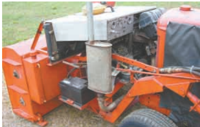
Snowblower is powered by a Volkswagen Golf 65 hp diesel engine equipped with a 5-speed transmission.
