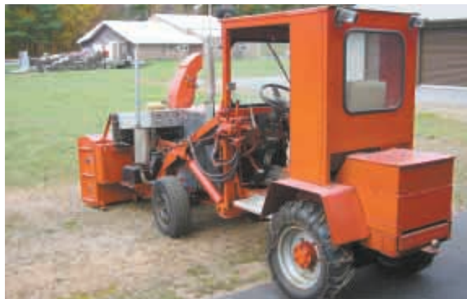
"It can handle snow up to 32 in. deep and throw it out up to 40 ft.," says Jeff Lang about his home-built tractor equipped with a loader-mounted snowblower.
