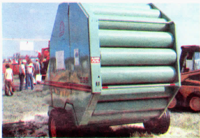
Owatonna's new model 595 big round baler is equipped with 21 rollers, each measuring 12 in. in dia.
