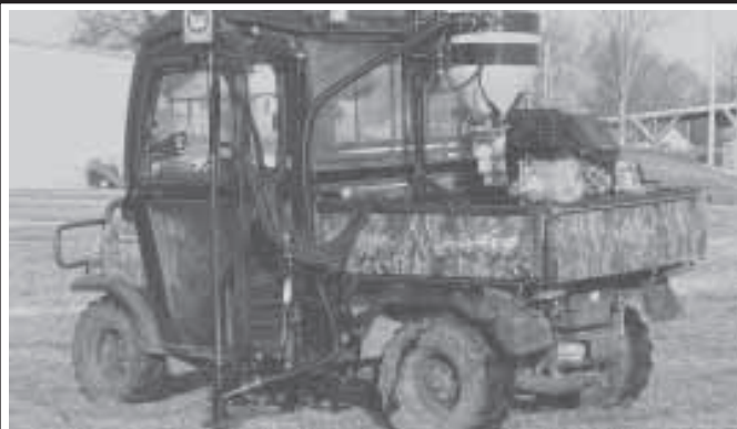
Vacuum-powered collection system is combined with Big John Mfg.'s Speedy Soil Sampler. Auger mounts on side of a pickup or ATV and gets down to a 36-in. depth.
