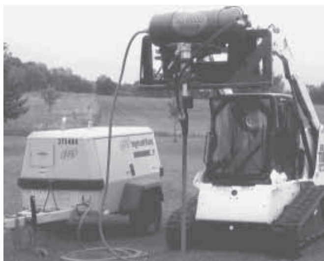
Soil Shaker is a skid steer attachment designed to loosen septic drain fields. It uses a 1 3/4-in. dia. pneumatic probe hammer to penetrate soil.
