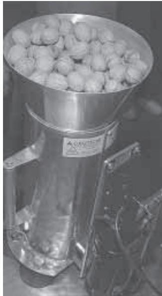
Nut cracker consists of a spinning cone inside a stationary cylinder. Nuts fall between the two, according to their width, and are cracked with even pressure.
