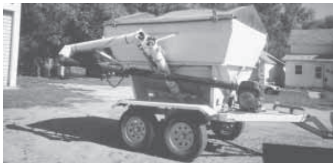
Ron Hanen converted this fertilizer cart to fill his bean planter. A gas engine is used to belt-drive a hydraulic pump, which operates a hinged auger that he added to one side.
