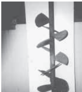
Ken Voigt figured out how to make an auger from paddles attached to a 1-in. dia. shaft.
