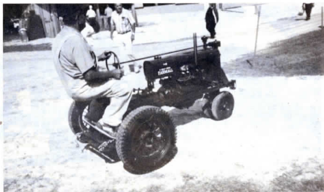
Erbe's Farmall is patterned after an F-20. It features a 3-speed transmission he built.
