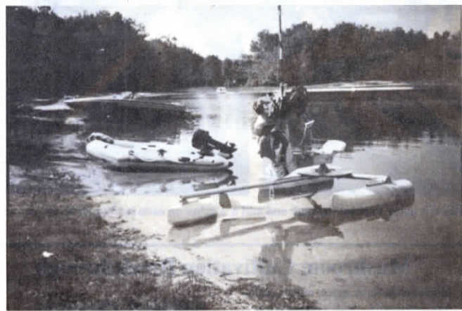
"Kiteboat" consists of frame and three floats. Pedals control winch and rudder.
