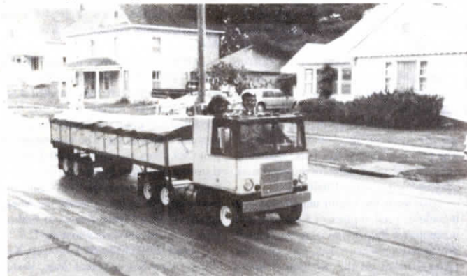
Mack CruiseLiner has 12-in. tires mounted on 4 by 8-in. rims, and a 13-ft. long trailer.
