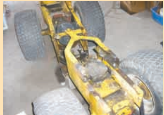
Tractor is powered by a Kohler engine from an old 1650 Cub Cadet (above). Its articulation point was based on the design used by Steiger tractors.
