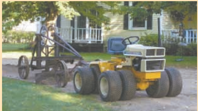
Darryl Schmidt used the rear axles from two 1970's Cub Cadets to build this dual wheel, articulated tractor.
