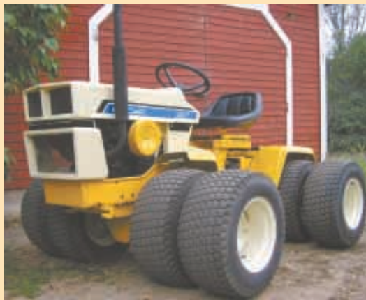
Darryl Schmidt used the rear axles from two 1970's Cub Cadets to build this dual wheel, articulated tractor.
