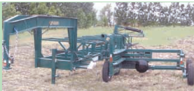
Hawkins Bale Flipper attaches to side of trailer and moves itself backward as each bale is loaded.
