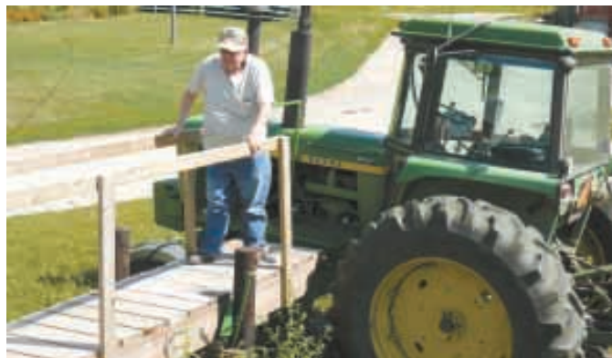
Nick Ruen built a wood ramp that lets Orrin Olson walk right into the tractor cab, without having to climb any steps.
