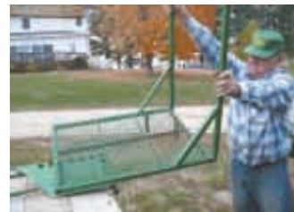
The Ruens also made a bigger entrance platform for the tractor that makes it easier to get in and out of the cab.
