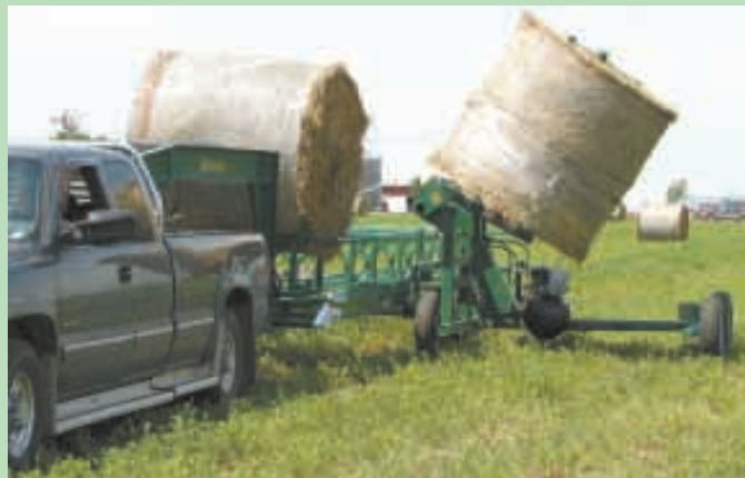
Loader is powered by an on-board motor and hydraulic pump and tows to field behind the bale trailer.
