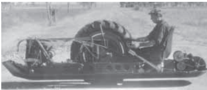
Designed many years ago, "motorized unicycle" could turn on a dime and travel narrow mountain trails.
