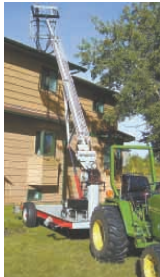
Boom raises basket up to 21 ft. A hydraulic cylinder can be used to extend basket out another 4 ft. "The 21-ft. lift height is enough that I can step out of the basket directly onto my house's roof," says Verbeek.
