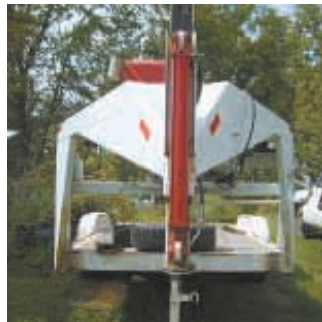
Mark Lockhart added hydraulics to the hitch on his gooseneck trailer, allowing him to easily tip up the trailer's front end and winch stuff on.
