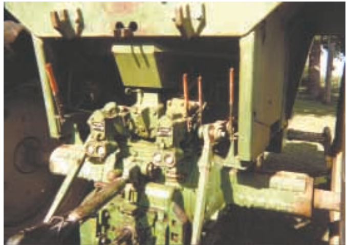
Willard Dittmer retrofitted his Deere 4230 with rear pto and throttle control.
