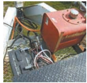
Mark Lockhart added hydraulics to the hitch on his gooseneck trailer, allowing him to easily tip up the trailer's front end and winch stuff on.
