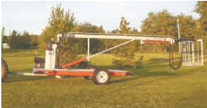
Dale Verbeek's home-built cherry picker mounts on a 2-wheeled trailer and is equipped with three hydraulic cylinders, all operated by a 1 hp electric motor.
