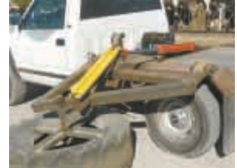
Greg Nye’s pickup-mounted “feed pusher” keeps feed in reach of cattle.
