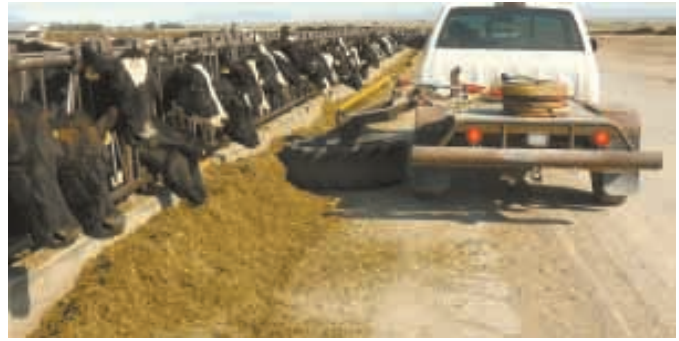
Greg Nye’s pickup-mounted “feed pusher” keeps feed in reach of cattle.
