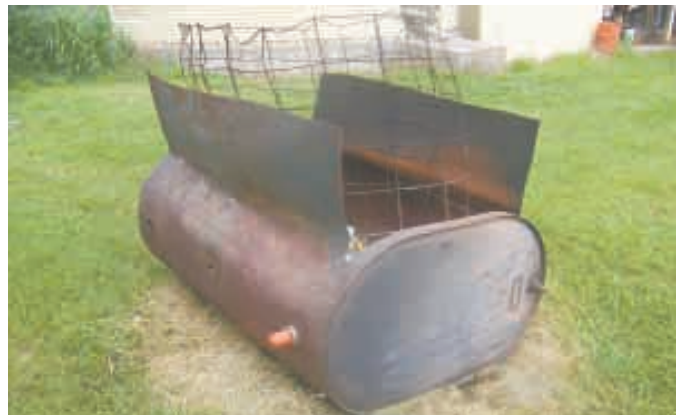
“I use it to burn seed corn sacks and other miscellaneous garbage,” says Kevin Holst, who converted an old 250-gal. fuel oil tank into this trash burner.
