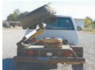
Greg Nye’s pickup-mounted “feed pusher” keeps feed in reach of cattle.
