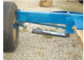
Beeliner anti-sway bar kit takes the sway out of trailing wagons.
