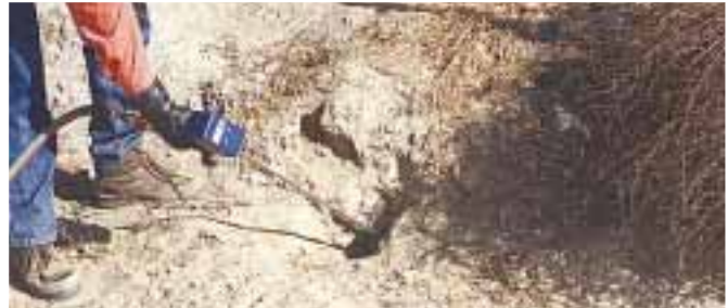
New gopher getter consists of a slender hand-held 36-in. long stainless steel probe that pumps a fumigant down into underground dens.
