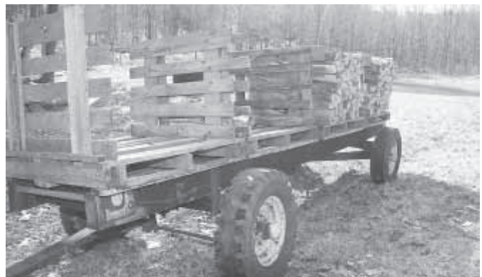
Pallet trailers are made from old hay wagons with the floorboards removed.
