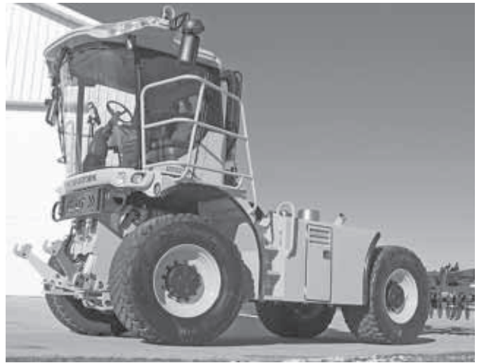
“Power Platform” is a 4-WD, 4-wheel steer rig that can be equipped with front and rear 3-pt. hitch, pto, and hydraulic outlets. It rides on 5-ft. high flotation tires.
