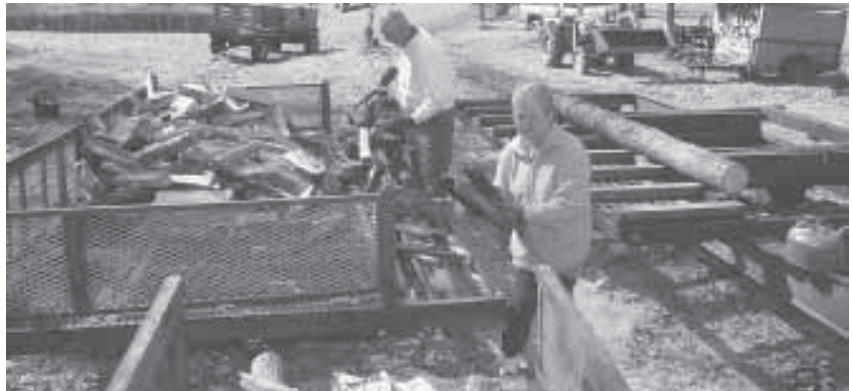
William Kelsey and his wife use eight different trailers to get wood back to their farm. Their splitting trailer is shown at left side of photo, and log-cutting trailer at right. Splitter mounts on wheels that roll down a pair of channel iron tracks. Note spaced cutting blocks on log-cutting trailer.
