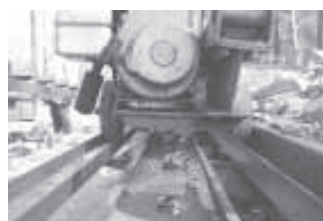
Log splitter rolls back and forth on tracks.
