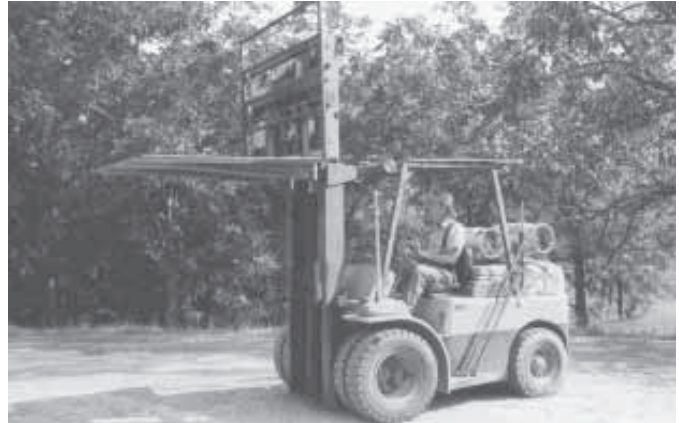
Work plate fits over forklift forks, allowing O.H. Rutledge to pick up an engine or other heavy object off the ground. Note how supports under plate are cut at an angle so it can slip plate under loads.
