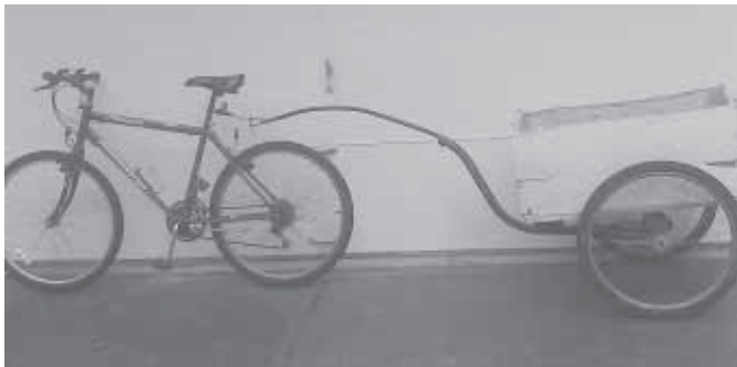
Cart rides on bike wheels and can be pulled with a mountain bike.
