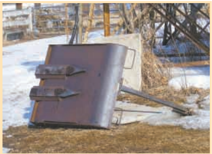
Points are welded on the bottom about 18 in. apart to make the tracks.
