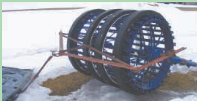
Ski trail groomer uses 34-in. dia. wheels fitted with thick urethane rings to make grooves in the snow for skis to follow.
