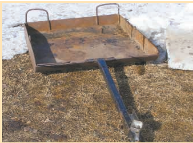
Sled-type "track setter" is a steel toboggan pulled by a snowmobile.
